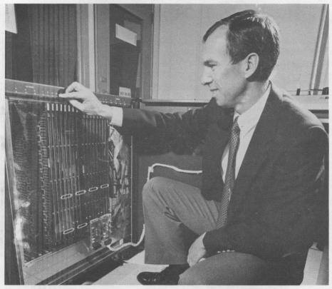
to show that Amdahl's Law is not a major barrier to solving computational problems if they're sized in proportion to the number of processors used. Here, Gil shows as much as can be readily seen of the 1024-processor hypercube computer on which his team achieved the recent breakthrough in massively parallel processing.
